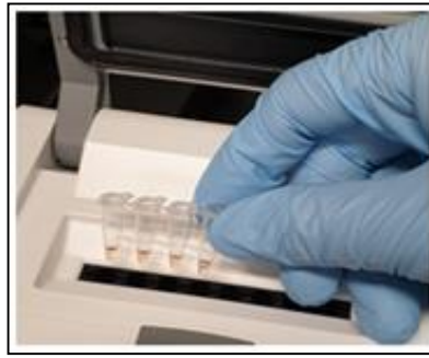
RNA-included LAMP Premix inserts to the Block of LAMP Device
