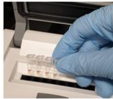
(2) Place the RNA Premix in PCR Device
