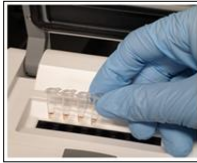
2. Insert RNA-included Premix to the Block of LAMP Device
